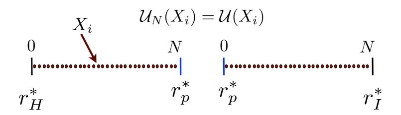
• To implement the PwP scheme numerically we use **PSCM**. Each subdomain is discretised with a number N of collocation points of a Lobatto-Chebyshev grid:
