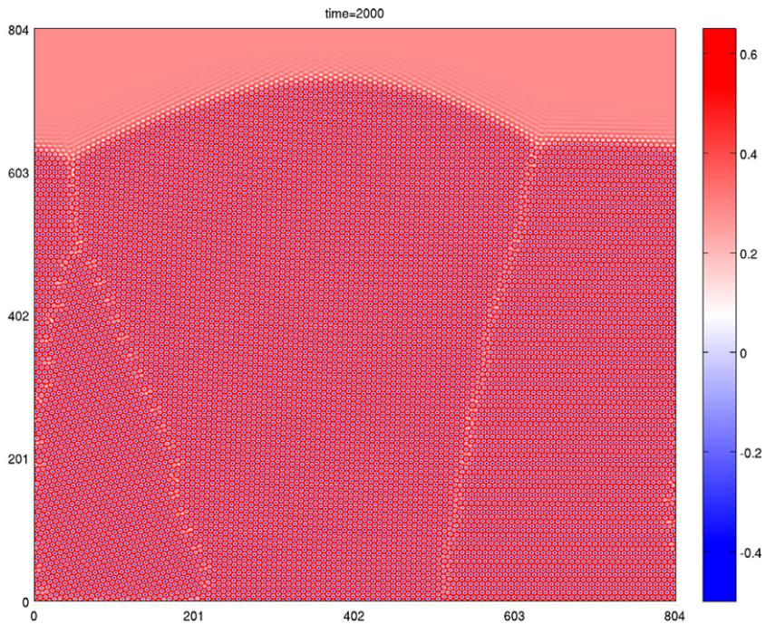
Fig. 7(b). Heterogeneous nucleation of three crystallites in a supercooled liquid. The snapshot shows the density field \phi at time t = 2000 . The parameters are \bar{\phi} = 0.285 , \epsilon = 0.25 , s = 1 , and h = 0.4 (2048 grid points in each direction). The second-order scheme (37) is used in the calculation.
