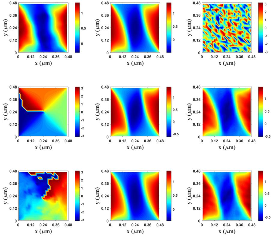
**Fig. 2.** Stable structures in the absence of magnetic field at 2ns when  $\alpha = 0.01, 10, 40$ . The color denotes the angle between the first two components of the magnetization vector. Top: Proposed method; Middle: GSPM; Bottom: SIPM. Left:  $\alpha = 40$ ; Middle:  $\alpha = 10$ ; Right:  $\alpha = 0.01$ . (For interpretation of the colors in the figure(s), the reader is referred to the web version of this article.)
