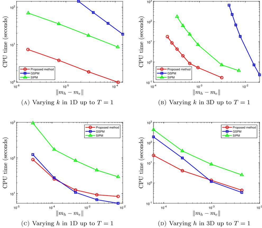
**Fig. 1.** CPU time needed to achieve the desired numerical accuracy, for the proposed method, the GSPM and the SIPM, in both the 1D and 3D computations. The CPU time is recorded as a function of the approximation error by varying  $k$  or  $h$  independently. CPU time with varying  $k$ : proposed method < SIPM < GSPM; CPU time with varying  $h$ : proposed method  $\approx$  GSPM < SIPM.
