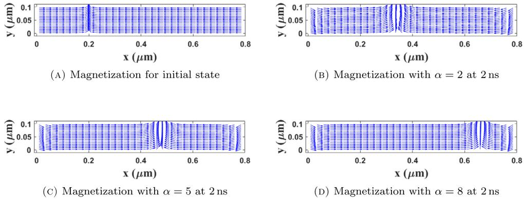
Fig. 5. Magnetization profiles of Neel wall motion in the presence of a magnetic field  $\mathbf{h}_e = 5$  mT, with  $\alpha = 2, 5, 8$  at 2 ns for the proposed numerical method. The in-plane arrow denotes the first two components of the magnetization vector. The wall moves faster for larger values of  $\alpha$  and its velocity depends linearly on  $\alpha$ .
