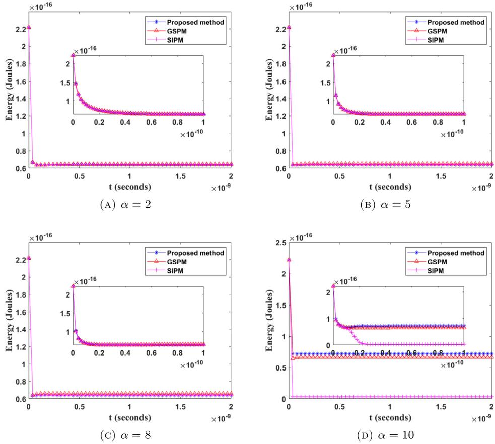
Fig. 4. Energy evolution curves in terms of time, for the numerical results created by three numerical methods up to  $t = 2$  ns in the absence of external magnetic field for (a)  $\alpha = 2$ , (b)  $\alpha = 5$ , (c)  $\alpha = 8$ , and (d)  $\alpha = 10$ . The energy dissipation pattern of the proposed method is consistent with the other two methods for (a), (b), and (c), and the SIPM has a slightly different energy dissipation pattern from the other two methods for (d).
