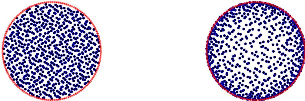
Figure 8: **Left:** A subset of 721 Halton points inside a unit disk is used as RBF inner nodes. In addition, 154 boundary points are distributed equally on the perimeter. **Right:** The Halton points are clustered toward the boundary with a mapping function  $\tilde{r}_i = \sin(\frac{\pi}{2}r_i)$ . The boundary points are left intact.
